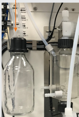
Buffer vessel outlet
